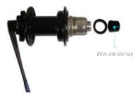
1C. Insert the 12mm Allen wrench into the non-drive side (left) with one 17mm open ended cone wrench on the drive side (right) and the drive side end cap should come off.
