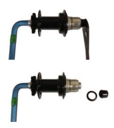
1D. Once the drive side end cap is off, pull hard to remove the freehub body. Clean and inspect the pawls/drive ring.
