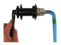
**2E.** Apply a small amount of Loctite 242 or 243 Blue to drive side end cap or shaft threads and re-install.
